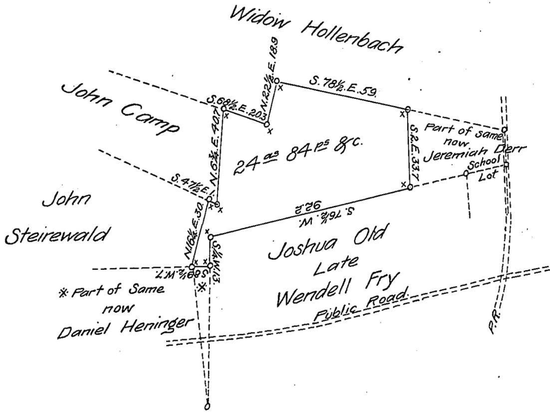
Draft of a tract of land situate in Weisenberg and Lynn townships, Lehigh County, Containing 24<sup>ac</sup> 84<sup>ps</sup> and allowance, surveyed for Joshua Old, the 22<sup>d</sup> day of Nov<sup>r</sup> A.D. 1872, being part of a larger tract of 41<sup>ac</sup> 80<sup>ps</sup> & allowance, originally surveyed in pursuance of a Wt. granted to Henry Sunday, dated the 31<sup>st</sup> day of Jan'y 1771.
